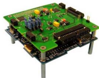
Space constraints meant that fine pitch connectors were required for the Delfi C3 project.
