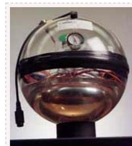
The glass optical modules, each the size of a bowling ball are arrayed on 19 cables set deep in the ice.
