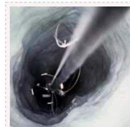
500 meter deep wells were drilled into the ice with the help of high-pressure hot-water drills.
