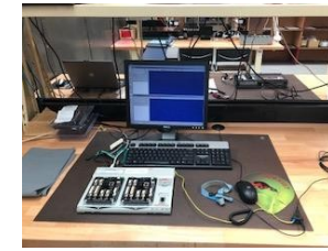
Cable Tester Station
