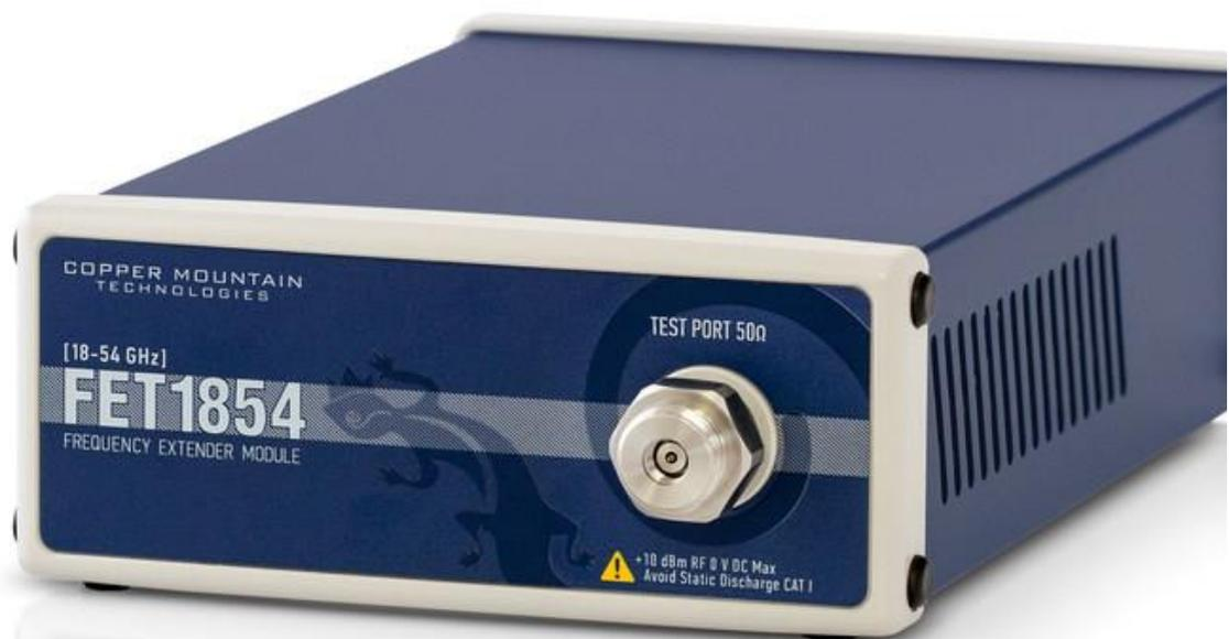
With the launch of the new FET1854 extenders, the CobaltFx system will allow engineers to build a scalable and affordable 5G testing solution. Anchored by a 2- or 4-port 9 or 20 GHz USB vector network analyzer, CobaltFx includes extenders in multiple frequency bands: 18 to 54 GHz, 50 to 75 GHz, 60 to 90 GHz and 75 to 110 GHz. Frequency extension is a standard software feature.
