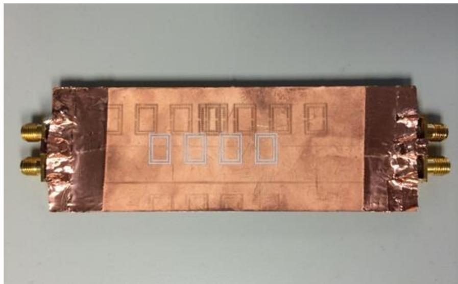
Figure 4 - Experimental common-mode Filter using split ring resonators designed by student Sang Goo under Dr. Ed Wheeler at Rose-Hulman Institute of Technology.
