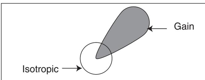
Figure 10: Antenna Gain
