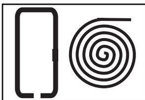
Figure 15: PCB Antennas
