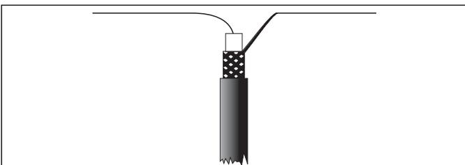
Figure 3: Basic Antenna
