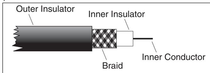
Figure 1: Typical Transmission Line
