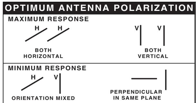
Figure 11: Antenna Polarization
